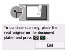
If you continue scanning, load the original on the platen and start scanning.
