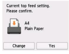
If the paper loaded in the top feed matches the paper information displayed on the printer's touch screen, select **Yes**.
