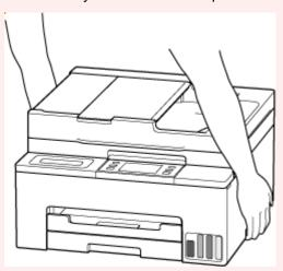
• After transporting your printer, place it in the original position, turn the ink valve lever to the left, and then turn on the printer.
