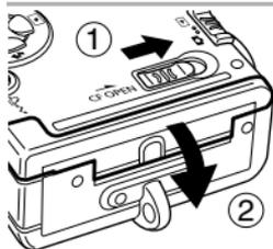
**1** Slide the lock up and open the CF card slot cover.
