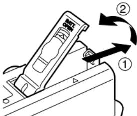
**1** Slide the battery cover in the direction of the arrows.
