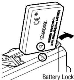
**2** Press the battery lock while inserting the battery pack all the way in until the lock clicks.
