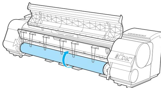
**7** Holding the Roll Holder flange (a), remove the holder from the Roll Holder Slot.
