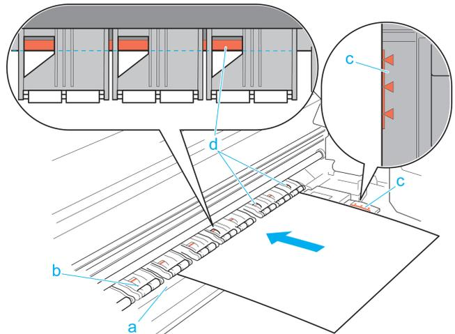
When inserted, sheets are automatically held by suction against the Platen.
