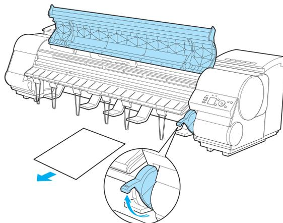
**6** Lower the Release Lever and close the Top Cover.
