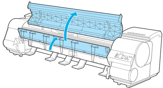
**3** Remove the six Ejection Supports and lower the Ejection Guide.
