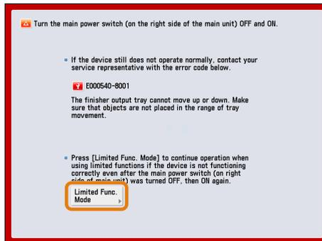
If [Limited Functions Mode] is displayed, you can temporarily set the Limited Functions Mode to continue to use the machine until the cause of the malfunction is cleared. For more information, see "Setting the Limited Functions Mode from the Service Call Message Screen," on p. 255.
