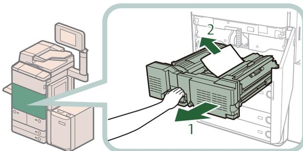
1. Grip the green lever, and pull out the fixing transport unit.
