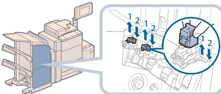
1. Pull out the empty staple case, holding it by its left and right sides.
