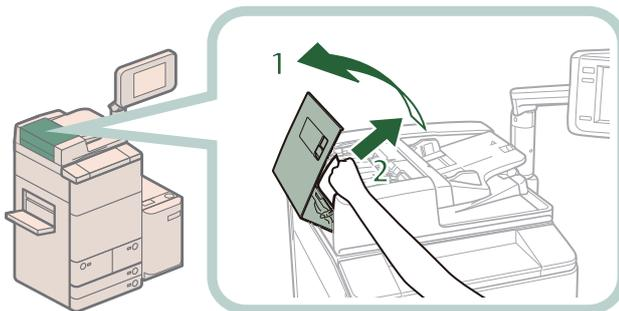
1. Pull the lever, and open the feeder cover.
