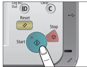
If the following screen appears, press **Start** to scan the next original. After all of the originals are scanned, press [Start Copying].
