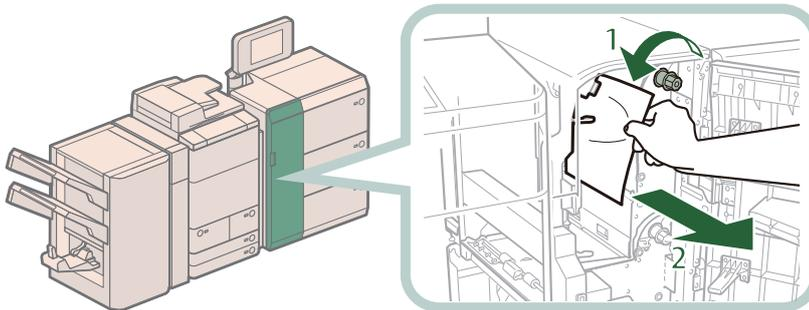
1. Turn the dial (D-A2) in the direction of the arrow (counterclockwise).
