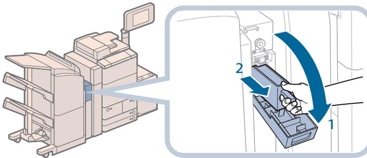
1. Open the front cover of the puncher.
