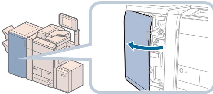
**2** Below the stapler unit is the staple waste tray. Pull out the staple waste tray.
