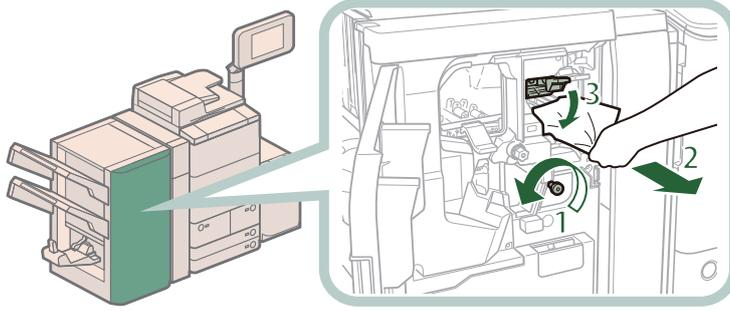
1. Turn the lower dial (F-C3) in the direction of the arrow (counterclockwise). Jammed paper is fed to the guide (F-C2).
