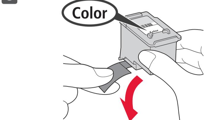
3 Unpack the FINE Cartridge, then remove the protective tape.
