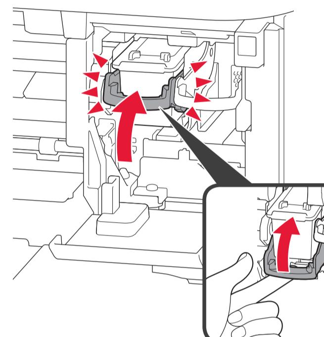
5 Lift the Ink Cartridge Lock Lever.
