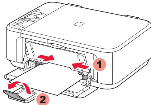
**4** Adjust the Paper Guide to fit the paper size used, then open the Output Tray Extension.
