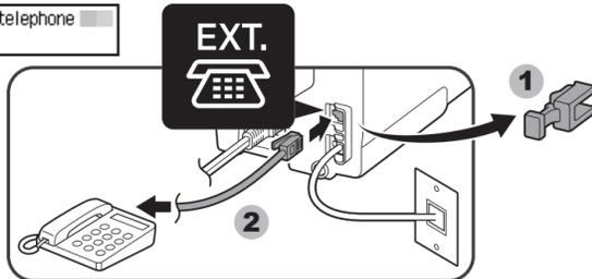
If you want to connect a telephone or an answering machine, remove the Cap, connect a telephone or an answering machine with a telephone line cable and press the **OK** button.
