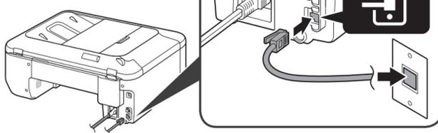
Connect the machine to a telephone jack with the supplied telephone line cable, then press the **OK** button.
