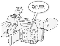
2 Press the POWER SAVE button to return the camcorder to record pause mode.
