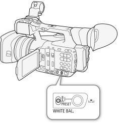
Custom white balance: You can use a white object to establish the white balance and set it to one of two custom white balance positions, A or A or B. These correspond, respectively, to positions A and B of the WHITE BAL. switch.
