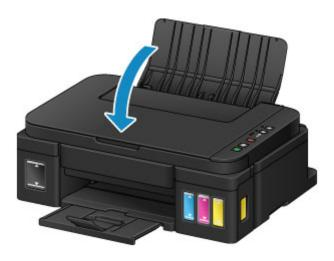
• After loading the original on the platen glass, be sure to close the document cover before starting to copy or scan.
