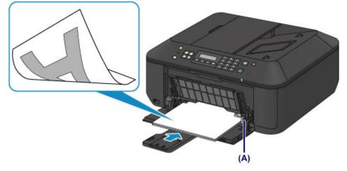
(4) Slide the right paper guide (A) to align the paper guides with both sides of the paper stack.
