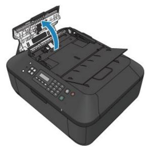
3. With a soft, clean, lint-free and dry cloth, wipe off any paper dust from the inside of the document feeder cover (A).
