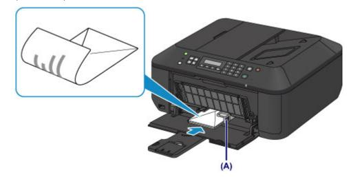
(4) Slide the right paper guide (A) to align the paper guides with both sides of the envelopes.
