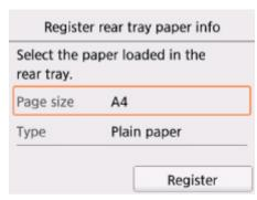
Register the paper size and the media type according to the loaded paper.
