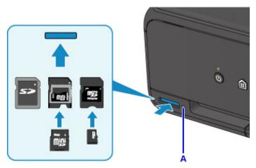
Be sure to attach the card adapter to the following types of memory card before inserting to the card slot.
