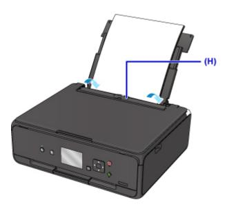
After closing the feed slot cover, the paper information registration screen for the rear tray is displayed on the LCD.
