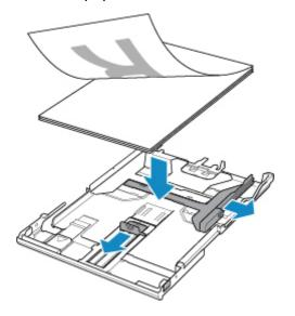
5. Align the paper guides (D) with the paper length and width.
