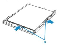
6. Mount the cassette cover, and then insert the cassette into the printer.
