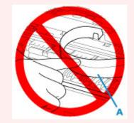
If you soil or scratch this part by touching it with paper or your hand, it could damage the printer.
