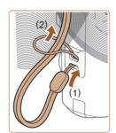
• Thread the end of the strap through the strap mount (1), and then pull the other end of the strap through the loop on the threaded end (2).
