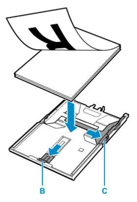
4. Align paper guides (B) in front and (C) on right with paper length and width.
