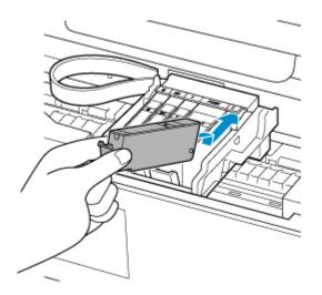
8. Press on the top of the ink tank until the ink tank snaps firmly into place.
