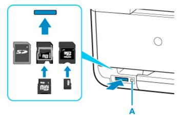
\* Be sure to attach the card adapter to the following types of memory card before inserting to the card slot.
