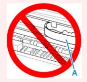
If you soil or scratch this part by touching it with paper or your hand, it could damage the printer.
