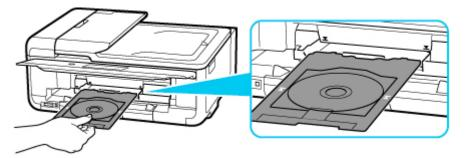
Insert multi-purpose tray straight in in horizontal direction until arrow (∑) on multi-purpose tray guide is approximately aligned with arrow (∑) on multi-purpose tray.
