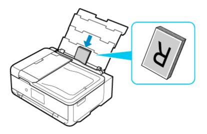
**5.** Slide right paper guide (D) to align with both sides of paper stack.
