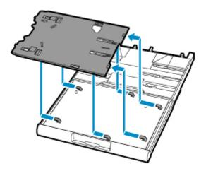
**12.** Open multi-purpose tray guide (L) and completely press it down.
