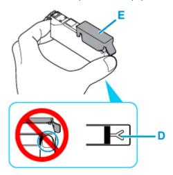
6. Lift up the tab on the orange protective cap (E) to remove it off GENTLY.
