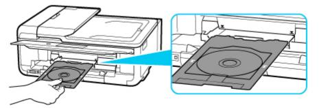
**16.** Insert multi-purpose tray straight in in horizontal direction until arrow (**∑**) on multi-purpose tray guide is approximately aligned with arrow (**∑**) on multi-purpose tray.
