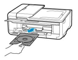
**19.** While pressing down lock (K), take out printable disc from slits (L) on multi-purpose tray, and remove it.
