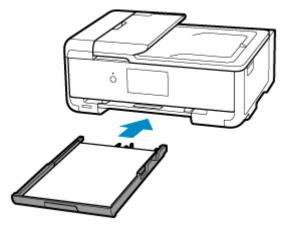
After inserting the cassette into the printer, the paper setting confirmation screen for the cassette appears on the touch screen.
