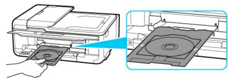
5. Insert multi-purpose tray straight in in horizontal direction until arrow (𝒴) on multi-purpose tray guide is approximately aligned with arrow (і) on multi-purpose tray.
