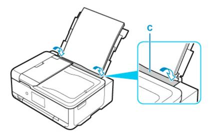
After closing the feed slot cover, the paper setting confirmation screen for the rear tray appears on the touch screen.
