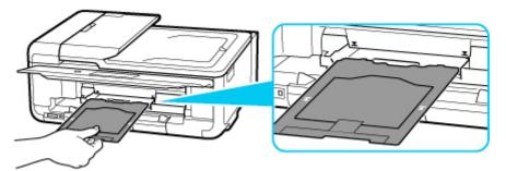
Insert multi-purpose tray straight in in horizontal direction until arrow (∑) on multi-purpose tray guide is approximately aligned with arrow (
