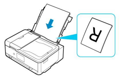
6. Slide right paper guide (D) to align with both sides of paper stack.
