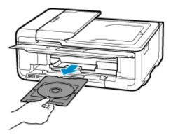
**2.** While pressing down lock (A), take out printable disc from slits (B) on multi-purpose tray, and remove it.
