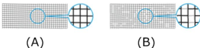
(A) As long as the horizontal lines are in line, and not missing, the nozzle is working normally.
