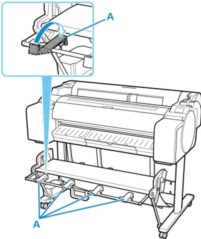
2. Hold onto the basket handle (A) and pull the basket release lever (B) towards you.
