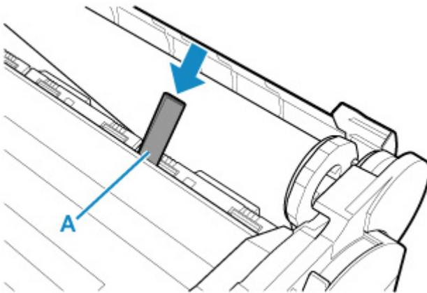
5. Remove scrap when it is pushed out onto platen.
