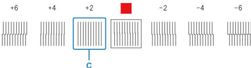
Example 2: Move the angle adjustment lever to a position between the numbers or between the number and the square (D) of the two sets of lines that are least misaligned. In this case, select -1.
