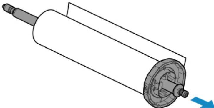
3. To remove 3-inch paper core attachment, press tabs (A) inward and remove attachment.
