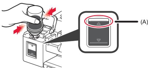
7 Replace the tank cap securely.
