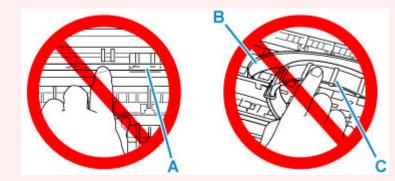
If you soil or scratch this part by touching it with paper or your hand, it could damage the printer.
