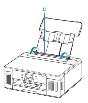
After closing the feed slot cover, the paper information registration screen for the rear tray appears on the LCD.
