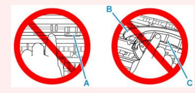
If you soil or scratch this part by touching it with paper or your hand, it could damage the printer.
