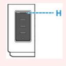
8. Once ink reaches the upper limit line, remove the ink bottle from the inlet.
