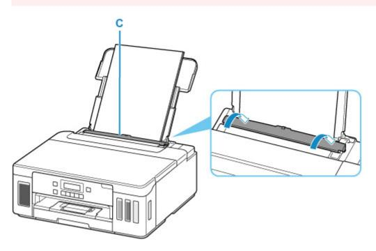
After closing the feed slot cover, the paper information registration screen for the rear tray appears on the LCD.
