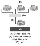
Use a highly shielded Category 5e or higher STP (Shielded Twisted Pair) Gigabit Ethernet cable.
