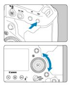
When you press a button such as  $\langle MODE \rangle \langle DRIVE AF \rangle \langle B \rangle$ , or  $\langle ISO \rangle$ , the respective function remains selectable for approx. 6 sec. ( $\bigcirc 6$ ). During this time, you can
