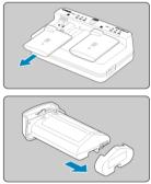
Remove the included protective covers from the charger and battery.
