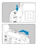
When you press a button such as  $\langle MODE \rangle \langle DRIVE \cdot AF \rangle \langle BOR \rangle$ , or  $\langle ISO \rangle$ , the respective function remains selectable for approx. 6 sec. (O6). During this time, you can turn the  $\langle AF \rangle \langle BR \rangle$  and the setting.
