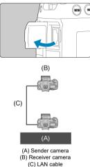
When using multiple receiver cameras, connect a LAN cable from the Ethernet terminal of the sender and receiver cameras to a hub. Up to 10 receiver cameras can be connected.
