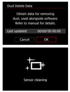
After the automatic self-cleaning of the sensor is performed, a message will appear. Although there will be a mechanical sound of the shutter during the cleaning, no picture is taken.
