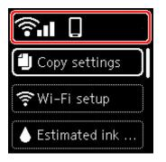
If the icon appears on the LCD, it indicates that Wi-Fi is enabled and the printer is connected to the wireless router.
