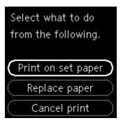
Use the  $\blacktriangle$   $\blacksquare$  buttons to select the appropriate action and press the printer's **OK** button.
