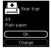
If the page size on the LCD matches the size of the paper loaded in the rear tray, select **OK**. If not, select **Change** to change the setting in accordance with the size of the loaded paper. • When you insert the cassette:
