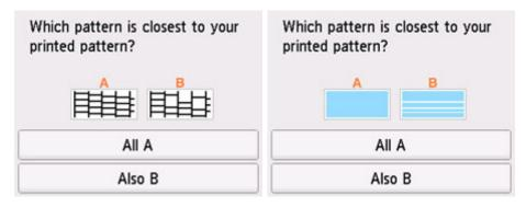
For A (no missing lines or no horizontal white streaks) in both the pattern C and pattern D:
