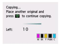
Load the original on the platen and press the same button (**Color** button or **Black** button) as the one which you previously pressed.
