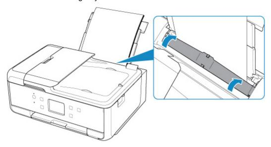
After closing the feed slot cover, the paper setting confirmation screen for the rear tray appears on the touch screen.
