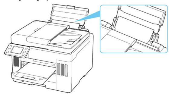
3. Remove foreign object by hand with paper inserted.
