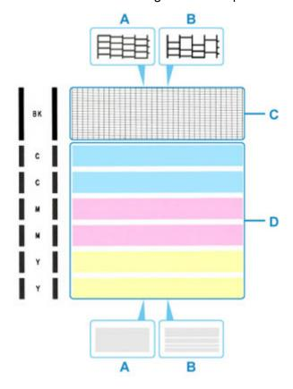
A: No missing lines/No horizontal streaks
