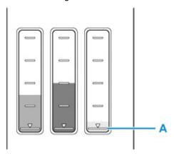
If you use the printer until the ink tank becomes empty, perform ink flush after refilling the ink tank.
