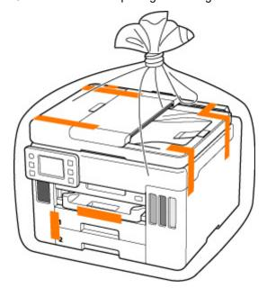
**10.** Attach the protective material to the printer when packing the printer in the box.
