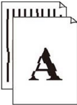
Lines Are Misaligned/Distorted
