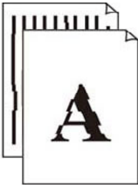
Lines Are Misaligned/Distorted
