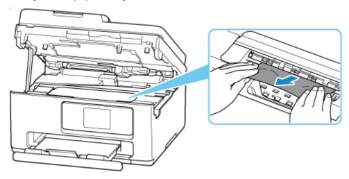
If the paper is rolled up, pull it out and grasp the edges of the paper.
