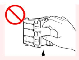
• Put the used one immediately into the plastic bag that came with the new maintenance cartridge and seal the bag by tying the opening tightly to prevent the ink from leaking.
