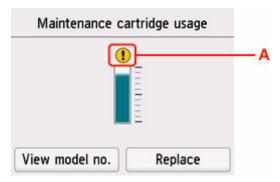
• The maintenance cartridge is almost full. Replace the maintenance cartridge as soon as possible.
