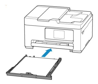
After inserting the cassette into the printer, the paper setting confirmation screen for the cassette appears on the touch screen.
