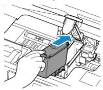
**2.** Close the ink cartridge locking cover to secure the FINE cartridge.
