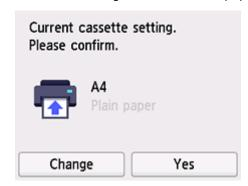
If the page size on the touch screen matches the size of the paper loaded in the cassette, select **Yes**. If not, select **Change** to change the setting in accordance with the size of the loaded paper.
