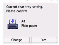
If the page size on the touch screen matches the size of the paper loaded in the rear tray, select **Yes**. If not, select **Change** to change the setting in accordance with the size of the loaded paper.
