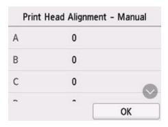
**9.** Examine first patterns and tap **A**. Select the number of the pattern in column A in which streaks/lines are least noticeable.
