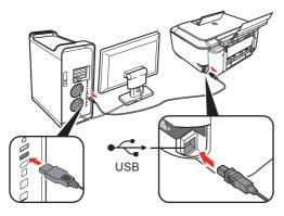
Connect one end of the USB cable to the computer and the other to the machine.
