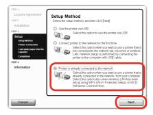
On the **Setup Method** screen, select **Printer is already connected to the network**, then click **Next**.
