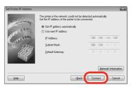
When the **Set Printer IP Address** screen appears, click **Connect**.
