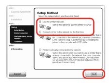
On the **Setup Method** screen, select **Use the printer via USB**, then click **Next**.
