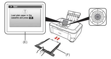
Confirm the message on the LCD (E), then load plain paper into the Cassette (F) and press the  $\bf OK$  button.
