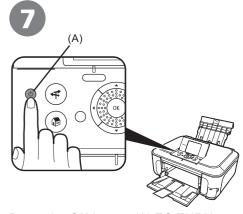
Press the **ON** button (A) TO TURN OFF THE MACHINE, then place the machine in the location where you will use it, and turn on it.
