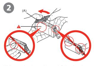
While pressing down with your left thumb, twist off the orange protective cap (A) located on the bottom of the ink tank.
