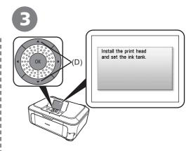
Use the ▲ or ▼ button (D) on the Operation Panel to select the language for the LCD, then press the **OK** button. The standby screen is displayed.
