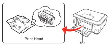
The Print Head is placed inside of the Paper Output Tray (A).
