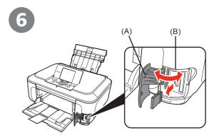
After printing, open the Card Slot Cover (A), pinch the memory card and pull it straight out, then close the Card Slot Cover (A).
