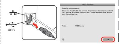
When the Setup Completion dialog box appears, remove the USB cable, then click OK.
