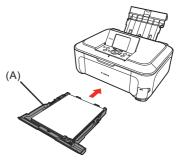
Insert the Cassette (A) into the machine until it clicks into place.
