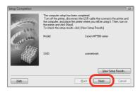
When the Setup Completion dialog box appears, remove the USB cable, then click Next.
