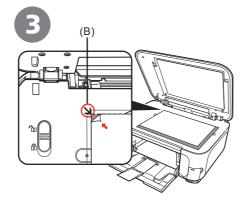
Place the document face-down and align it with the Alignment Mark (B).
