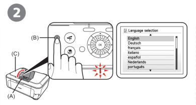
Open the Operation Panel (A), then press the ON button (B) to turn on the machine.
