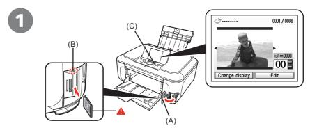
While the standby screen appears, open the Card Slot Cover (A), insert a memory card into the Card Slot, then close the Card Slot Cover (A).
