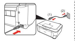
Plug in the power cord on the left side at the back of the machine and connect the other end to the wall outlet.
