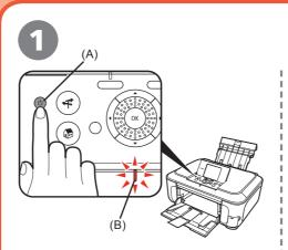
Press the **ON** button (A) to TURN OFF THE MACHINE.
