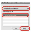
On the Canon IJ Network Scanner Selector screen, select Canon MP980 series Network in TWAIN Data Source Name and the MAC address of the machine in Network Device List, then click Apply to use the machine as a scanner.
