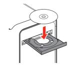
Turn on the computer, then insert the *Setup CD-ROM* into the CD-ROM drive.
