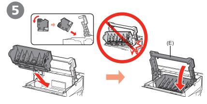
Tilt the Print Head and set it in place. Lower the Print Head Lock Lever (E) completely.
