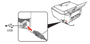
When the **Printer Connection** screen appears, connect the machine to the computer with a USB cable, then turn on the machine.
