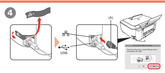
Connect the machine to the network device with a LAN cable (A), then click Yes.
