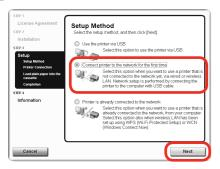
On the **Setup Method** screen, select **Connect printer to the network for the first time**, then click **Next**.
