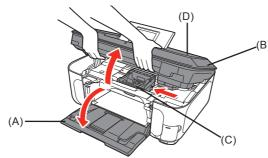
Open the Paper Output Tray (A), then lift the Scanning Unit (Cover) (B) until it locks into place.
