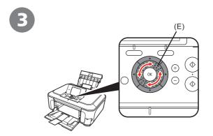
Rotate the Easy-Scroll Wheel (E) to display a photo to print.
