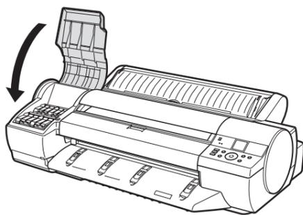
After all the ink tanks have been installed, the printer automatically starts charging the system with ink. Charging the system with ink for the first time takes about 20 minutes. Install the software and electronic manuals on your computer while charging the system with ink. If you install the software and electronic manuals later, wait until the system is charged with ink, and then proceed to "Load Paper to Adjust the Printheads" on page 11.
