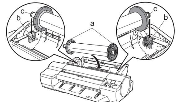
**Caution** • Be careful to not pinch your fingers between the axis of the roll holder (c) and the guide grooves (b) when loading paper.
