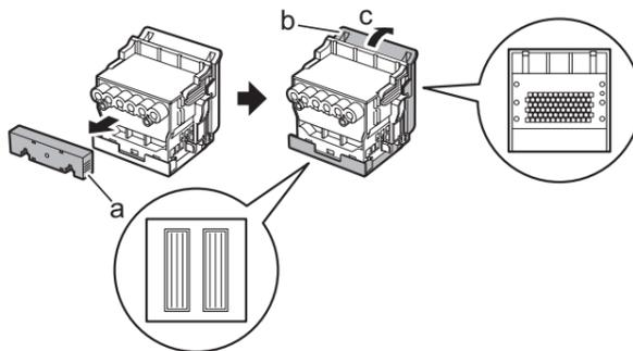
**9** Insert the printhead into the carriage (b) with the ink holes (a) up and facing the front of the printer as shown in the figure. Carefully push the printhead firmly into the carriage (b), ensuring that the parts that were covered by the protective parts do not touch the carriage (b).
