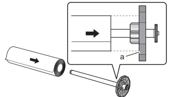
**4** Slide the holder stopper for the 2-inch paper core onto the roll holder from the left until its flange (a) is against the roll of paper.
