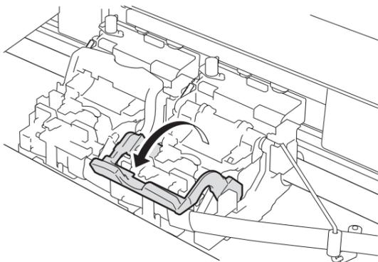
**6** Lift the printhead fixer cover to open it fully.
