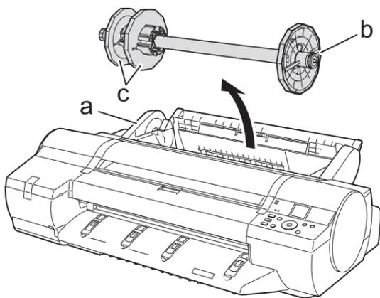
**5** Remove the orange tape on the top cover (a) and the ejection guide (b) and all the packing materials. After removing the orange tape and packing material from inside the ejection guide (b), reattach it.
