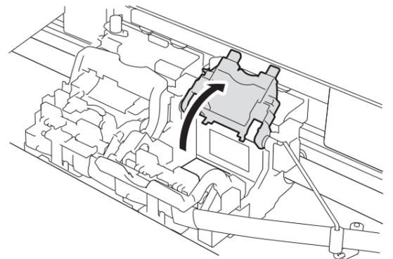
**7** Hold the printhead by the grips (a) as you remove it from the pouch.
