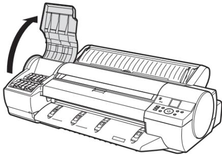
**2** While pressing the stopper of the ink tank lock lever inwards, open the ink tank lock lever upwards.
