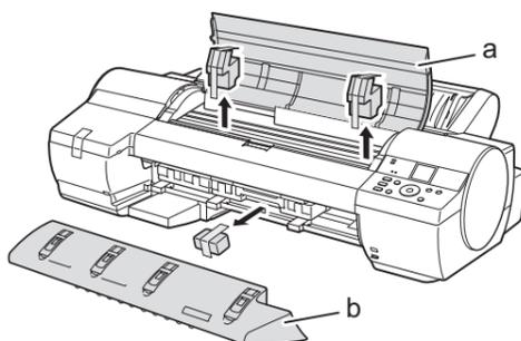
**6** Lift the belt stopper (b) from the carriage shaft (a) and pull it towards you to remove it.
