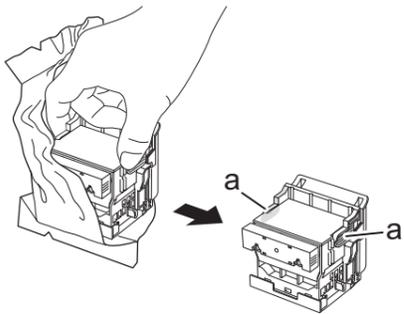
**8** Remove the orange protective part (a). To remove the other orange protective part (b), push the grip (c) as you remove it.
