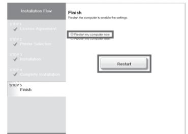
**14** When you restart the computer, the software settings are enabled. The software installation is now completed. An **iPFxxxx Support** desktop icon is created after installation. (iPFxxxx represents the printer model.)
