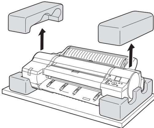
**3** At least three people are needed to lift the printer by its carrying handles (a), located under its right and left ends, and to place it on a table or other flat surface. The printer weighs 51 kg and requires at least three people to lift it by its carrying handles (a) under its right and left ends.
