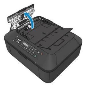
3. With the prepared cloth, wipe off any paper dust from the inside of the document feeder cover (A).
