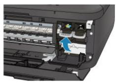
After confirming that the FINE cartridge is installed properly, close the paper output cover. If the problem is not resolved, remove the FINE cartridges, then install them again. Refer to <u>Replacing a FINE Cartridge</u> for how to install the FINE cartridges. • When copying, see also the sections below:
