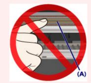
If the paper or your hands touch the clear film and blot or scratch it, the machine can be damaged.
