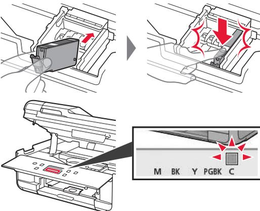
If the color is not displayed on the screen even though you have installed the ink tank, the color of the ink tank may be wrong or you may have installed an ink tank, such as one with a different model number, that is not supported by this printer. Either install an ink tank for the correct color or use the provided ink tank for setup.
