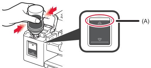
**7** Replace the tank cap securely.
