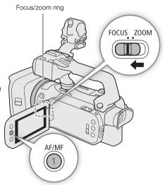
When manual focus is activated, you can register a certain focus point and then, after you focus manually somewhere else, have the camcorder return to the preset focus position.
