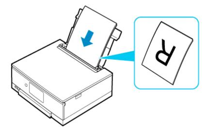
**6.** Slide right paper guide (D) to align with both sides of paper stack.
