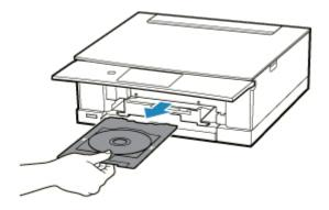
**17.** While pressing down lock (M), take out printable disc from slits (N) on multi-purpose tray, and remove it.
