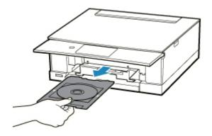
**18.** While pressing down lock (K), take out printable disc from slits (L) on multi-purpose tray, and remove it.
