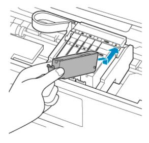
8. Press on the top of the ink tank until the ink tank snaps firmly into place.
