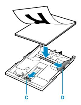
**5.** Align paper guides (C) in front and (D) on right with paper length and width.
