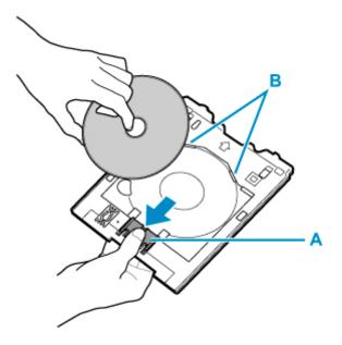
**3.** Insert multi-purpose tray straight into multi-purpose tray storage compartment. When not using the multi-purpose tray, store it in the multi-purpose tray storage compartment.
