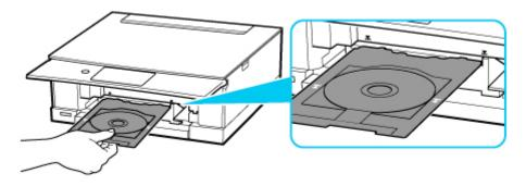
**14.** Insert multi-purpose tray straight in in horizontal direction until arrow (**▼**) on multi-purpose tray guide is approximately aligned with arrow (**△**) on multi-purpose tray.
