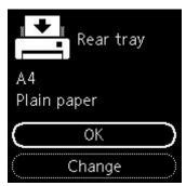
If the page size on the LCD matches the size of the paper loaded in the rear tray, select **OK**. If not, select **Change** to change the setting in accordance with the size of the loaded paper.
