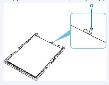
**6.** Slide front paper guide (C) to align it with paper stack.
