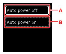
A: Specify the length of time to turn the printer off automatically when no operation is made or no printing data is sent to the printer.
