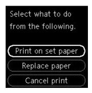
Use the  $\triangle$   $\nabla$  buttons to select the appropriate action, then press the printer's **OK** button.
