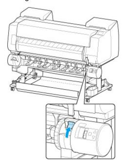
**7.** Hold flanges (A) so that roll holder's black gear is on left, align roll holder shaft with roll holder slot left and right guide grooves (B), and load.
