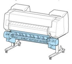
4. Refer to Printer Stand Setup Guide and attach basket to Stand.
