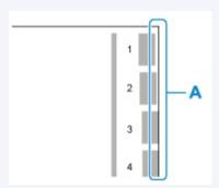
Check the edges (A) of the paper of No. 1 to No. 8 of the output pattern, and select the appropriate number for the amount of protrusion of the printed pattern.
