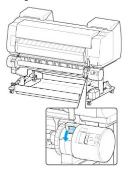
**9.** Change the feed flap switch on top of the roll unit so that the switch indicator (A) is aligned with ● (B) position on the take-up icon.
