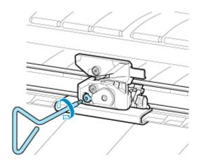
• After the cutter blade is secured, check that the cutter blade does not come off. If the cutter blade comes off, this may damage the printer.
