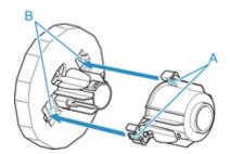
**5.** Insert the holder stopper into the Roll Holder, and then lock it in place.
