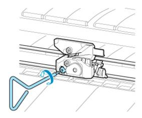
7. Remove cutter blade while holding D.
