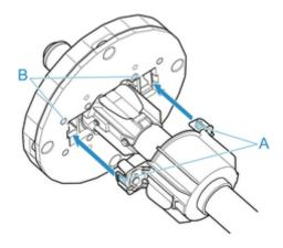
**3.** With leading edge of roll paper facing forward as shown, insert Roll Holder from right side of roll. Insert firmly until roll paper touches flange (A) of Roll Holder.
