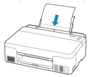
If the flashing **Paper** lamp and the size of the paper loaded in the rear tray are different, press the **Paper Select** button to switch.
