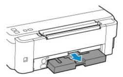
**6.** Lift the maintenance cartridge a little and pull it out.
