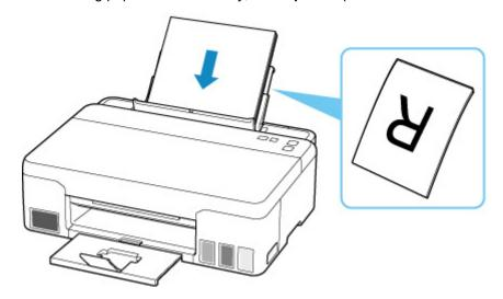
7. Slide right paper guide to align with both sides of paper stack.
