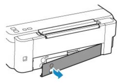
5. Pull out the maintenance cartridge until it stops.
