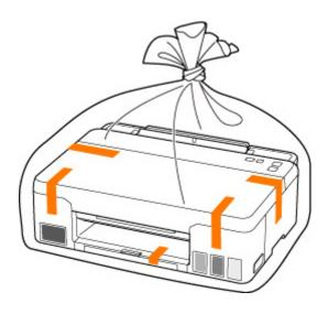
**11.** Attach the protective material to the printer when packing the printer in the box.
