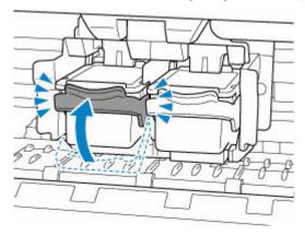
After confirming that the FINE cartridge is installed properly, close the cover.
