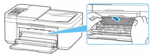
If the paper is rolled up, pull it out and grasp the edges of the paper.
