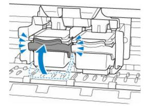
Make sure FINE cartridge holder motion is not impeded by stabilizer, jammed paper, etc.
