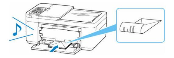
**5.** Slide the right paper guide to align both paper guides with both sides of the envelopes.
