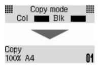
When the **COPY** button, **SCAN** button, **FAX** button, or **Setup** button is pressed, the display switches to copy mode, scan mode, fax mode, or setup menu screen.
