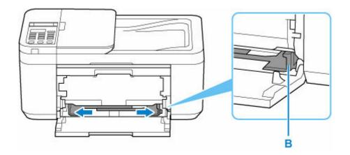
**4.** Load paper stack in portrait orientation WITH PRINT SIDE FACING DOWN, and place it in center of front tray.
