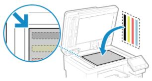
Place the print side of the correction image face down with the black band at the back of the machine.
