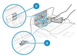
Wipe with a cloth soaked in water and wrung out. Next, wipe with a soft, dry cloth.
