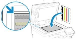
Place the print side of the correction image face down with the black band at the back of the machine.
