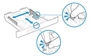
2 Align the projections on the paper guides with the size markings of the paper to be loaded.
