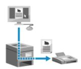
You can convert a document or photo to a black and white image and send it via a fax driver installed on a computer connected to the machine. You can send a fax in the same way as printing a document or photo from a computer. To send a fax, you do not need to prepare printed materials.
