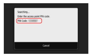
Once this screen is displayed, you must register the WPS PIN code to the wireless LAN router within 10 minutes.
