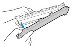
Be careful not to touch the drum surface on the bottom of the toner cartridge.
