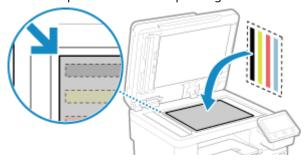
Place the print side of the calibration image face down with the black band at the back of the machine.
