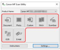
Click [ScanGear] to display ScanGear MF and configure the advanced scan settings. For more information, click [ ?? ] on ScanGear MF to display help.
