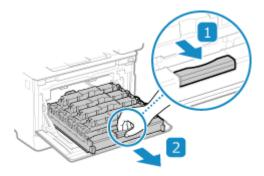
Pull the toner cartridge to be replaced straight up and out of the machine.
