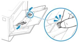
While pressing the lock release lever, move the paper guides.
