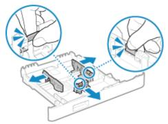
While pressing the lock release lever, move the paper guides.
