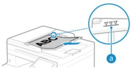
Make sure the placed originals do not exceed the load limit line (a). If they exceed the load limit line, there may be misfeeds or a paper jam.
