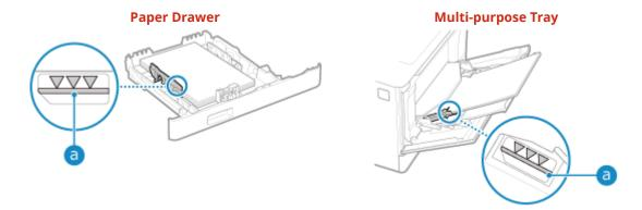
Check that the paper guides are aligned with the markings and are not too loose or too tight.
