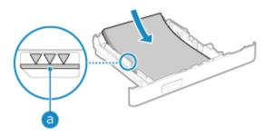
• Align the paper with the paper guide on the front side of the paper drawer.
