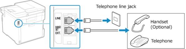
Connect the handset or telephone to the external telephone jack (EXT.) on the machine.
