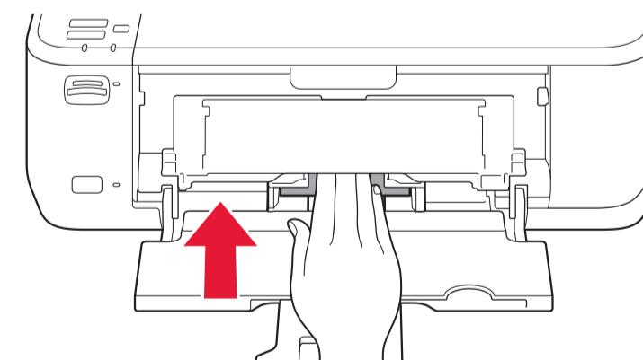
Insert paper with the **printable side down** until it stops. When using photo paper, machine settings for media type and size should be adjusted. For details, refer to the **On-screen Manual** which will be installed later.
