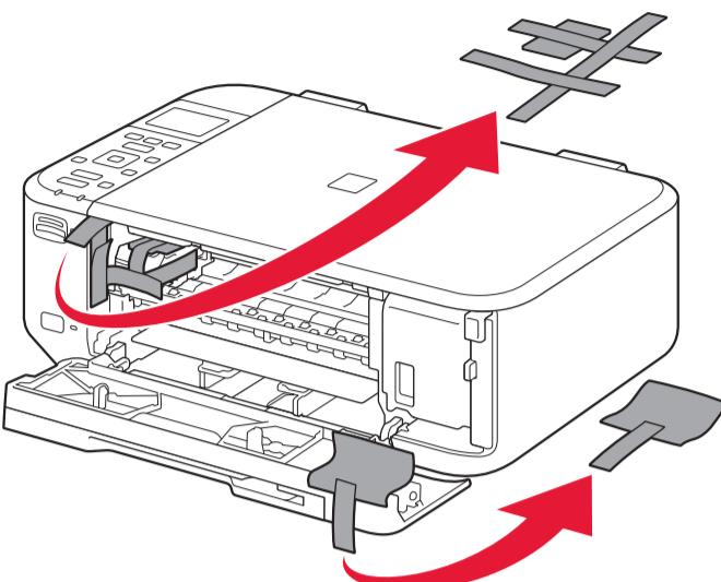
3 Remove the orange tape and protective material.
