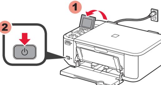
6 Adjust the angle of the LCD, then press the ON button.
