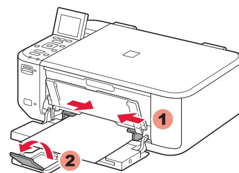
4 Adjust the Paper Guide to fit the paper size used, then open the Output Tray Extension.
