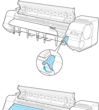
5 Holding the paper on both sides, pull the jammed portion out toward the front. Use scissors or a cutting tool to cut away the printed or wrinkled portion.
