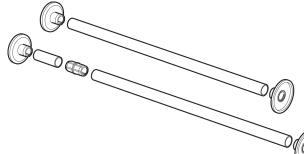
**16** Refer to the following table and securely insert the Weight Flange and Weight Joint suitable for the type and width of roll into the Weight Roll.
