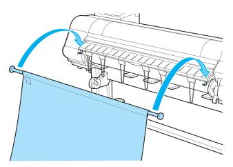
**6** Form the Basket Cloth into a sloping shape to make it taut, and attach the middle Basket Rod to the Rod Holder.
