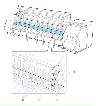
If paper dust has accumulated in the Vacuum holes (a) on the Platen, in the Borderless Printing Ink Grooves (b), or on the cutter guide (c), use the Cleaning Brush (d, provided with the printer) to wipe it away.
