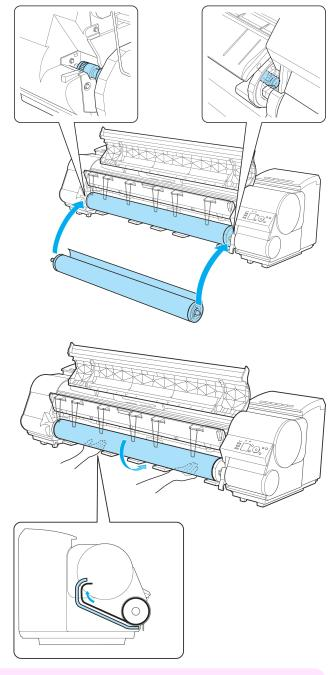
• When printing without borders, definitely set the blue Switch on the platen to the • side. If the switch is set incorrectly, print quality may deteriorate. (See "Setting the Blue Switch on the Platen.") —P.893
