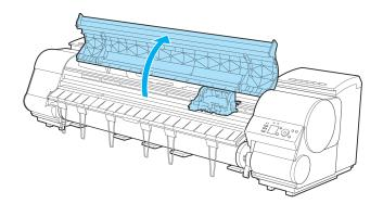
2 If the Cutter Unit or Carriage Cover is dirty, use a damp cloth that you have wrung out completely to wipe it clean.
