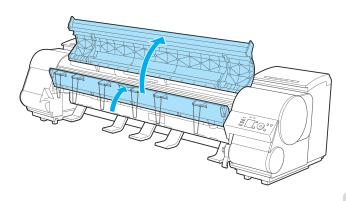
3 Remove the six Ejection Supports and lower the Ejection Guide.
