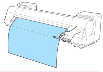
• Cut at the dotted line printed on the paper. If you cut on the printer side of the dotted line, the paper leading edge may rub against the printhead and may deviate from the paper retainer.
