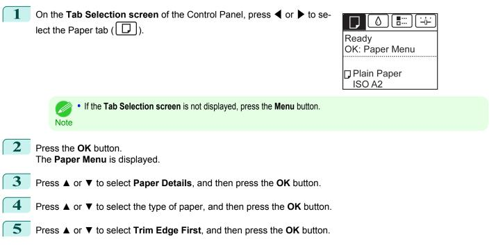
Press  $\blacktriangle$  or  $\triangledown$  to select the desired setting option, and then press the **OK** button. This setting takes effect the next time you load a roll.
