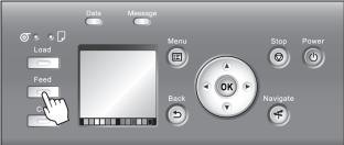
**9** Press  $\blacktriangle$  or  $\blacktriangledown$  to align the paper leading edge with the (a) position.
