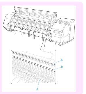
7 Holding the new Shaft Cleaner by the grips (a), attach it to the Carriage.
