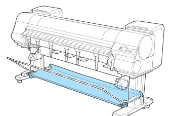
2 Remove the Output Stacker from the printer. Remove the front Basket Rod from the left and right basket arms, and remove the back Basket Rod and black cord from the Rod Holder.
