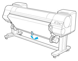
**12** Making sure the roll paper is not slack, tape the left and right side of the leading edge to the paper core.
