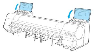
• Do not remove the Maintenance Cartridge except when the message for replacing it is displayed. If you remove the Maintenance Cartridge while ink is being drawn out, the ink may leak out.
