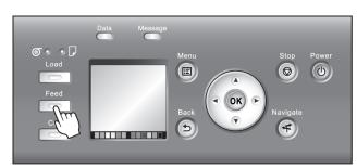
2 Hold down the ▼ button to advance the roll a little. To protect the paper that has been rewound, advance it an amount longer than the outer circumference.
