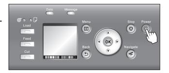
The **Power Lamp** is lit when the printer finishes starting up, and the printer is now in **Standby**.
