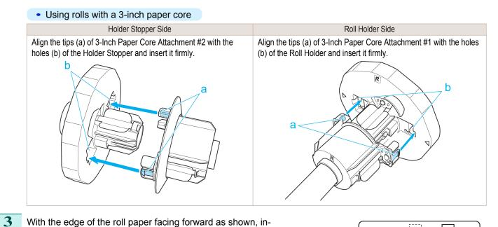
With the edge of the roll paper facing forward as shown, insert the Roll Holder from the right of the roll. Insert it firmly until the roll touches the flange (a) of the Roll Holder, leaving no gap.
