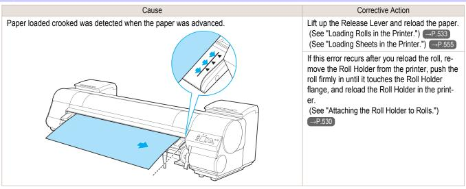
• To disable this message (if it is displayed repeatedly despite reloading paper, for example), choose Off or Loose in the Skew Check Lv. setting of the printer menu. However, this may cause jams and printing problems because paper may be Important askew when printed. Also, the Platen may become soiled, which may soil the back of the next document when it is printed.
