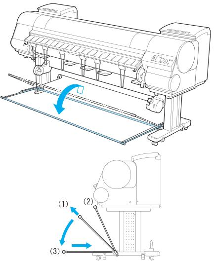
Using the output stacker for ejection in front
