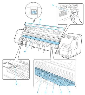
• Never use flammable solvents such as alcohol, benzene, or thinner. If these substances come into contact with electrical components inside the printer, there is a risk of fire or electrical shock.
