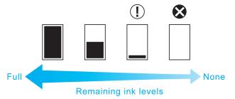
If the Display Screen indicates to replace the Ink Tank, replace the Ink Tank. If a message is displayed indicating to check the remaining ink levels, or after tasks that consume a lot of ink such as large-format printing or head cleaning, check the remaining levels and replace Ink Tank as needed. (See "Replacing Ink Tanks.")  $\rightarrow$  P.826
