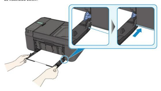
When the cassette is inserted properly, you hear an electric sound once.
