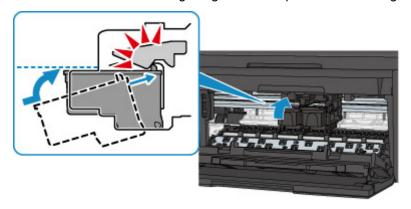
When the FINE cartridge is installed properly, you hear an electric sound once.
