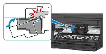
When the FINE cartridge is installed properly, you hear an electric sound once.
