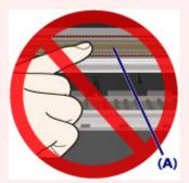
If the paper or your hands touch the clear film and blot or scratch it, the machine can be damaged.
