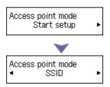
7. Check **SSID** information in the printer screen, then press the **Back** button (C).
