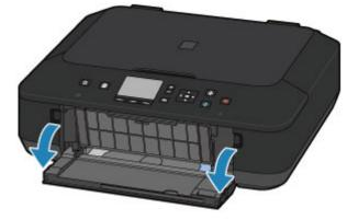
(2) Hold the right tab on the front tray to pull out the feeder until it stops.
