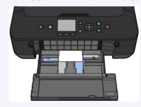
(6) Holding the right tab on the front tray, push the feeder back until the arrow (▷) on the front tray is aligned with the arrow (<) on the machine.
