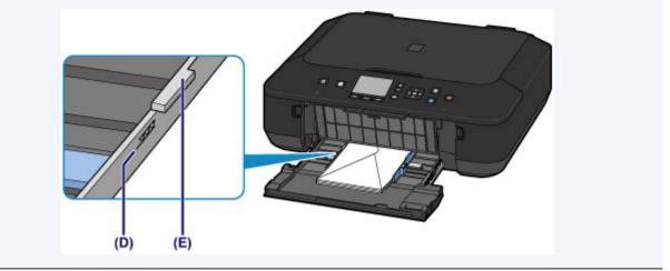
(6) Holding the right tab on the front tray, push the feeder back until the arrow (▷) on the front tray is aligned with the arrow (<) on the machine.</p>
