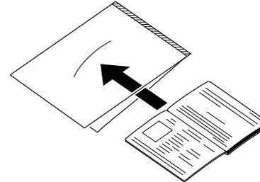
3. Load the document with the sealed end of the carrier sheet as the leading edge and the page you want to scan facing down. Adjust the document guides on both sides of the document after placing the document.
