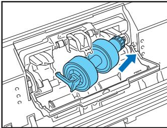
6. Push the left side of the retard roller to secure it to the scanner.
