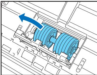
3. Remove any dirt from the roller using a cloth that has been soaked in water and thoroughly wrung out.
