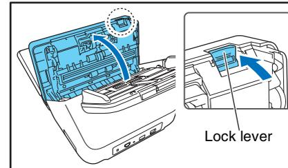
4. Pull out the jammed document in the direction that seems the easiest to remove it.
