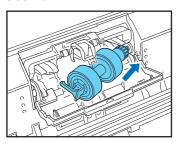
**6.** Push the left side of the retard roller to secure it to the scanner.
