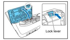
2. Use a commercially available air blower to remove any dust and paper particles that have accumulated inside the scanner.
