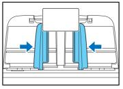
3. Place the card face down with the top edge at the bottom of the tray.
