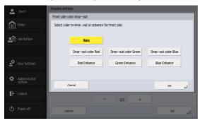
The color drop-out function has a "drop-out" effect that leaves out a specified color (red, blue, or green) while scanning, and a "color enhancement" effect that emphasizes a specified color. You can set each of these effects for the front side and back side.
