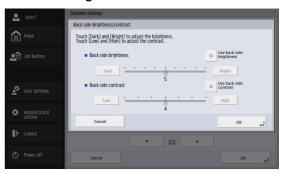
This is enabled when you scan both sides of a document and should be used when the document has front and back sides of different density. Select [Use back side brightness (contrast)] to change the settings for the brightness and contrast of the front and back sides of the document.
