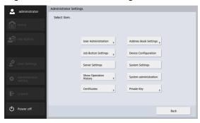
2. Press the [Device Configuration] - [ScanFront Maintenance] - [Roller counter reset] button to display the roller counter reset screen.
