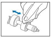
Install the cleaned retard roller by inserting the right side first.
