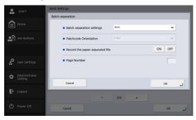
You can enable batch separation to be performed when a blank page or a patch code sheet is detected.
