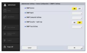
SNMPv1 determines the scope of communication with information called community names, but these names are passed on to the network in plain text, making them vulnerable to security breach. If you need to ensure security, disable SNMPv1 and use SNMPv3.
