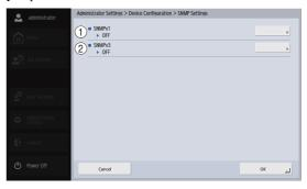
SNMP is a protocol for monitoring and controlling communication devices on a network based on a management information database (called MIB), and can be used to check the ScanFront status and error information using a PC. The ScanFront supports SNMPv1 and SNMPv3 with enhanced security capabilities, and you can use either or both. Set according to the purpose of use and environment.
