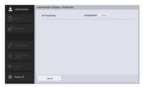
The private key is used when sending scanned images using SFTP. Use this menu to select the private key used in combination with the public key that were registered for public authentication of the SFTP server.
