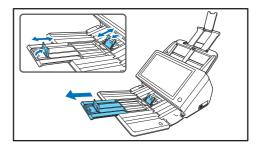
When scanning documents of different size at the same time, the scanned documents may not collect neatly on the eject tray. In such cases, scan with the tray extension extended.
