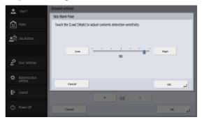
When [Skip Blank Page] is selected in the scanning side settings, this setting is enabled, and you can adjust the sensitivity level for skipping blank pages.
