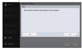
Confirm the message and press [Yes] to perform initialization, and the scanner will turn OFF.
