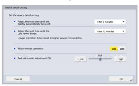
Adjust the wait time until the display automatically turns off.
