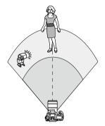
Fully automatic wireless flash photography using one receiver and one sender.
