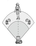
All flash units fire at the same output, and the total, combined output is automatically controlled to provide standard exposure.
