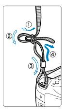
Pass the end of the strap through the camera's strap mount eyelet from the bottom. Then pass it through the strap's buckle as shown in the illustration. Pull the strap to take up any slack and make sure the strap will not loosen from the buckle.
