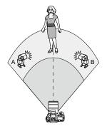
Receivers can be assigned as flash groups A and B, and you can adjust the relative output of each.
