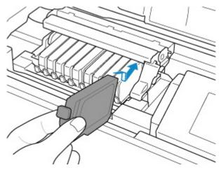
9. Press on the top of the ink tank until the ink tank snaps firmly into place.
