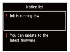
Use the  $\blacktriangle$   $\triangledown$  button to select a message and press the **OK** button to view the message details screen to check the details and take action.
