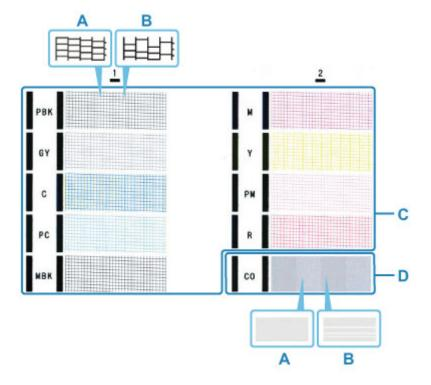
A: No missing lines/No horizontal streaks
