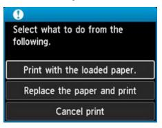
Select the appropriate action using the  $\Delta \nabla$  buttons and press the printer's **OK** button.
