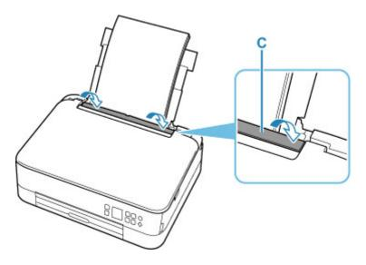
After closing the feed slot cover, the paper setting confirmation screen for the rear tray appears on the LCD.
